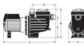
\* Suction and delivery accept 40mm PVC pipe on the I.D. and 50mm fitting on the O.D.
